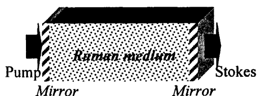
Fig.2 Structure of Raman laser
