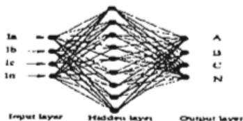
Fig.3. ANN consisting of four inputs, one hidden layer with five neurons and four outputs.
