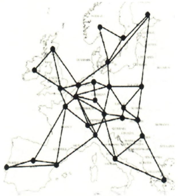
Fig. 5: Experimental physical network topology, COST266.
