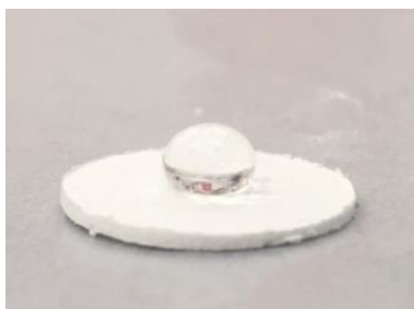
Figure 4. The hydrophobic property of marshmallow gel
