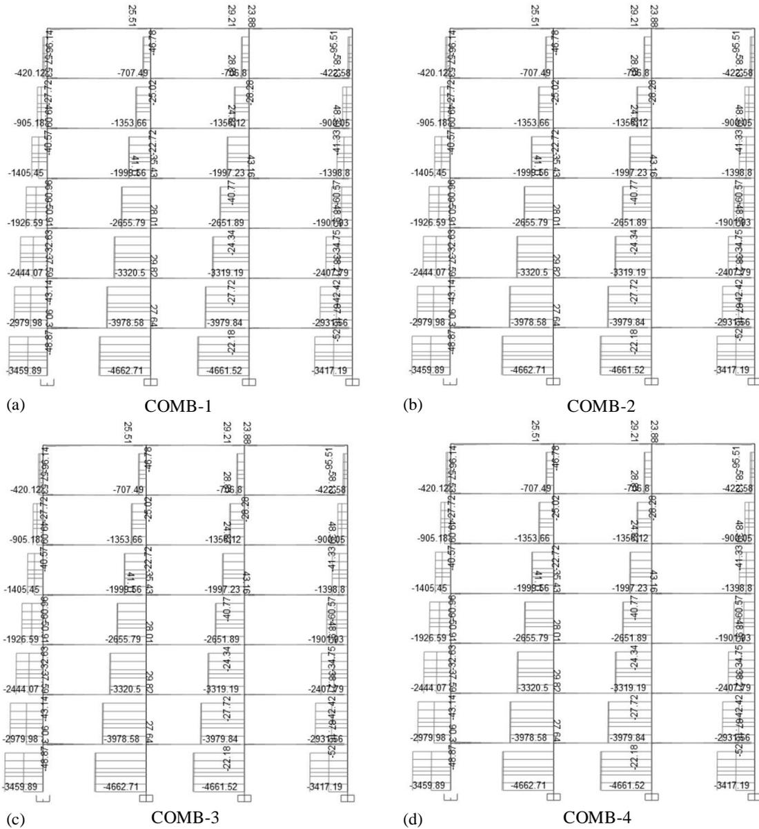
Fig. 8. Contribution of vertical ground motion on the axial response of structure subjected to load combinations.
