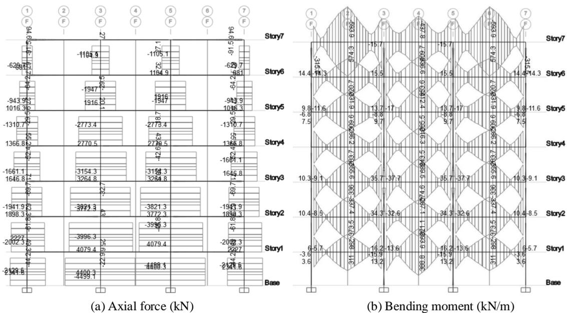
Fig. 4. Axial force and bending moment of building subjected to vertical ground motion (axis F).
