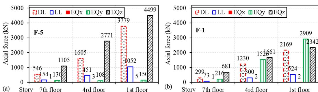
Fig. 6. Comparison of the axial force of RC building subjected to different loadings.
