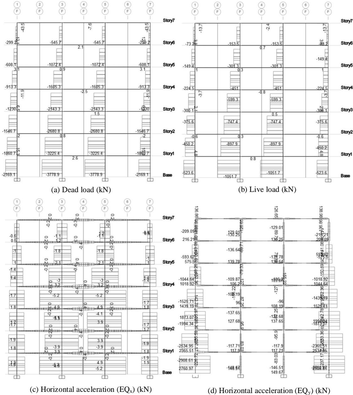
Fig. 5. Comparison of the axial force of RC building subjected to different loadings (axis F).
