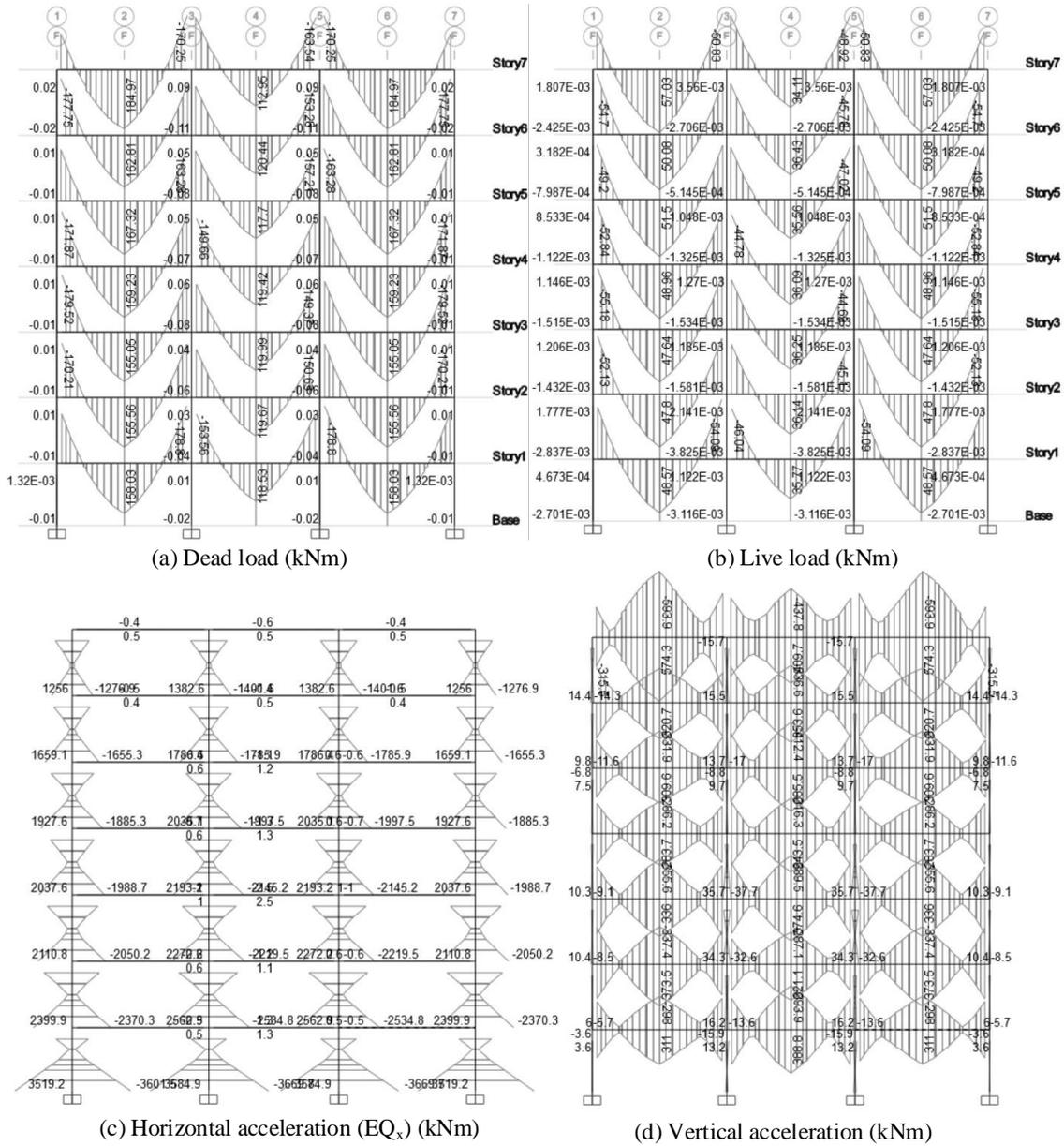
Fig. 7. Comparison of the bending moment of RC building subjected to different loadings.
