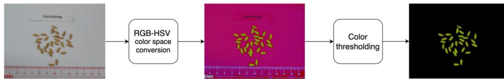
Figure 3. Workflow to separate rice grains from the input image background
