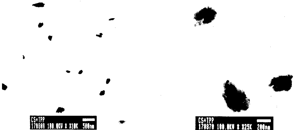
Fig.2: TEM photographs of non-loaded CS (left) and ART-loaded CS (right)
