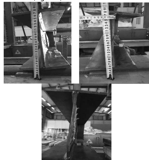
Figure 7. Failure mode of specimens M1, M2, M3
