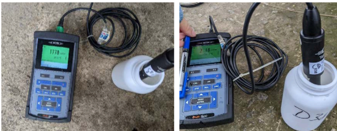
Figure 4. Investigate, examine, measure electrical conductivity, and collect samples in the field
