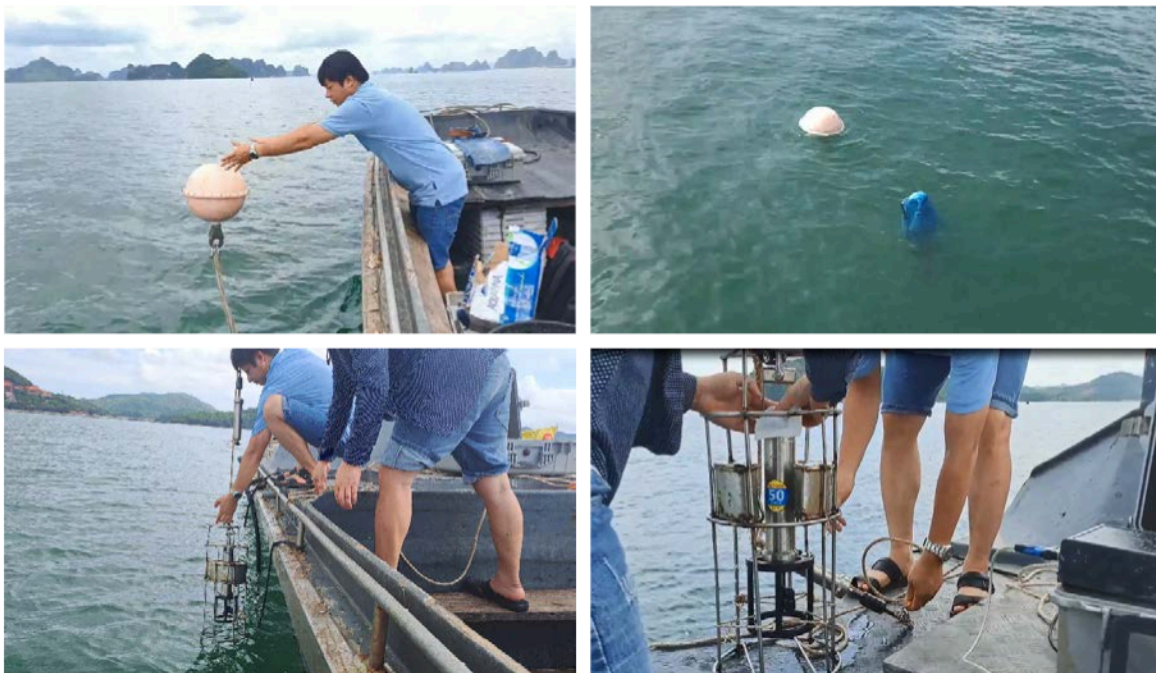
Figure 6. Set up the buoy and equipment to measure temperature and salinity, at sea of Van Don - Quang Ninh
