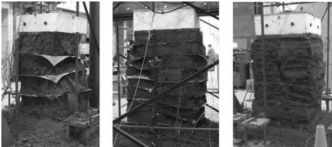
a. S_v \approx 16 inches b. S_v \approx 8 inches c. S_v \approx 4 inches.
