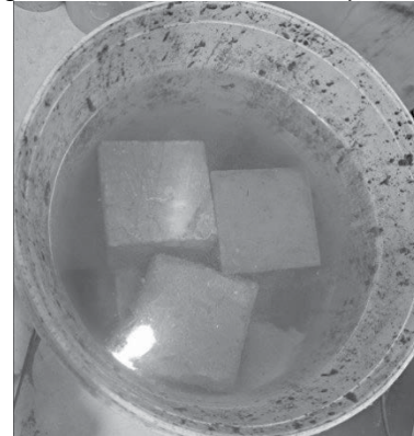
Figure 1. Concrete sample curing by water immersion
