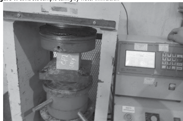
Figure 2. Concrete compression testing
