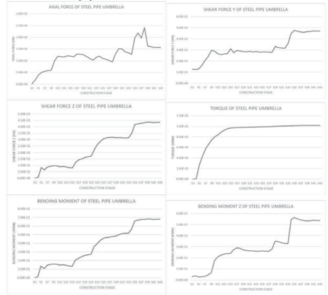
Figure 10. Forces and moment of steel pipe umbrella
